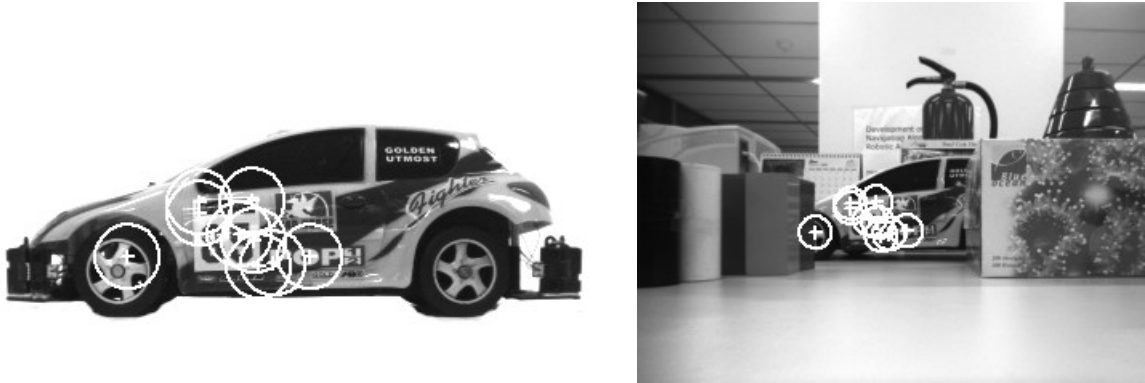
Fig. 8. Interest points automatically matched in a model image and a camera-captured view.
